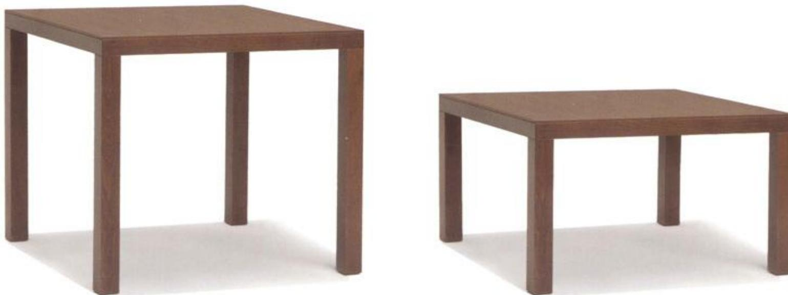
Table with four legs. Solid beech structure, 70x70 section legs, plywood top with beech veneer, mortise and tenon joints flush with outer edges. Top with finger and dowel joints. Anti-warping via lag screws reinforced with anchor bolts. Polyurethane spray finish.
