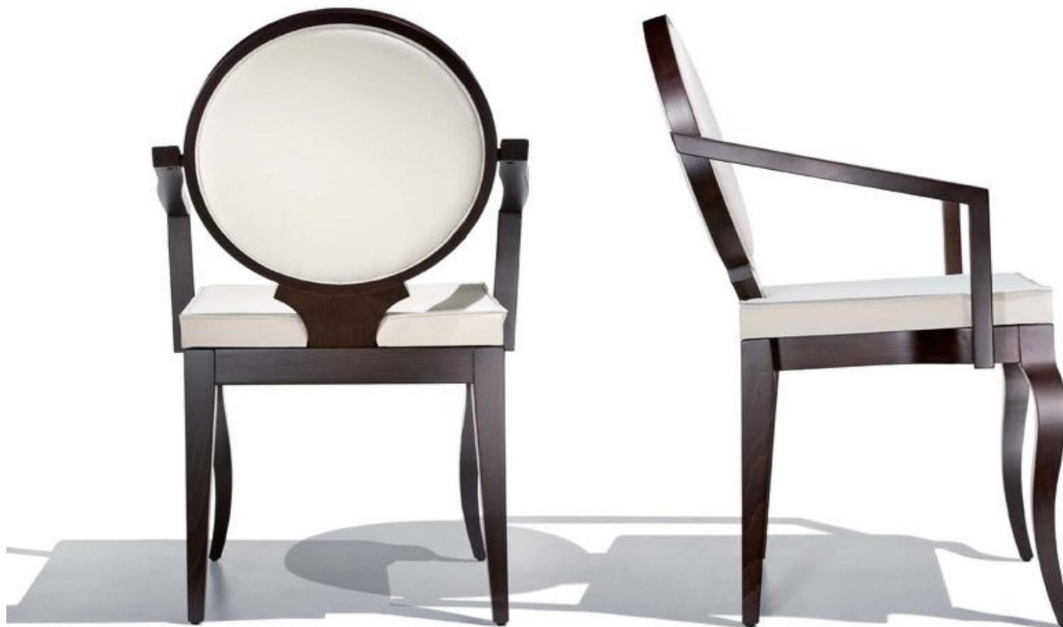
Chair with ash frame with mortise joints, backrest made of curved slats of ash, seat padded with 40 kg/m<sup>3</sup> density polyurethane foam. Seat panel made of birch plywood with high resistance paint finish.
